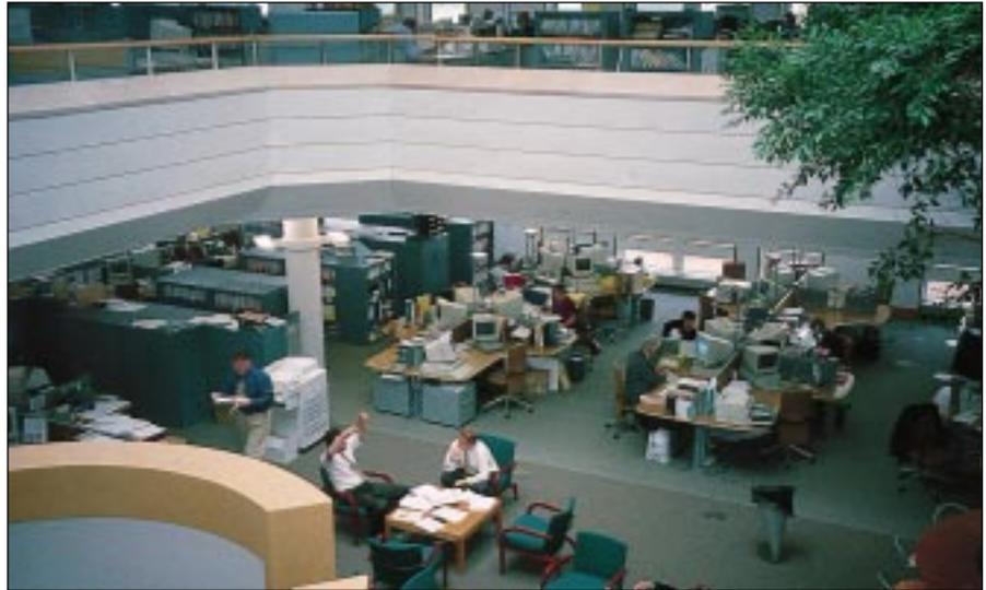
The ground floor offices at Co-operative Retail Services, viewed from an atrium. Due to the unreliable lighting control system, the metal halide uplighters tend to be on outside of normal office hours, contributing to an 'uplift' of 3-4°C to the supply air temperature in the first floor plenum.
