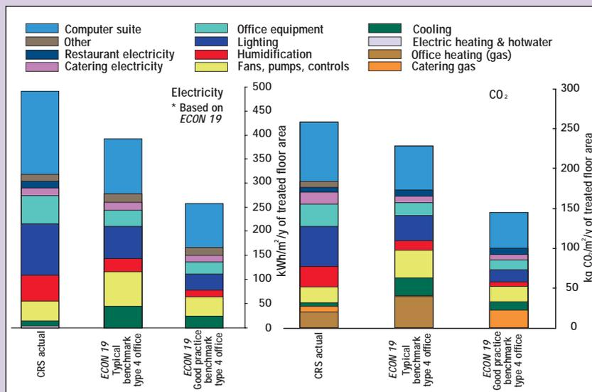
FIGURE 1: End-use energy breakdown at the Co-operative Retail Services headquarters building. The conversion factors are: gas – 0.2 kg CO<sub>2</sub>/kWh and electricity – 0.52 kg CO<sub>2</sub>/kWh.
