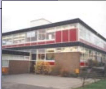
2. Lights on, blinds down – and wonky: a variation on a well-worn theme particular to school buildings. This is evidence that good façade detailing – inclusive of window design, solar shading, blinds and window opening mechanisms – must be very carefully integrated to optimise daylighting and ventilation control strategies.
