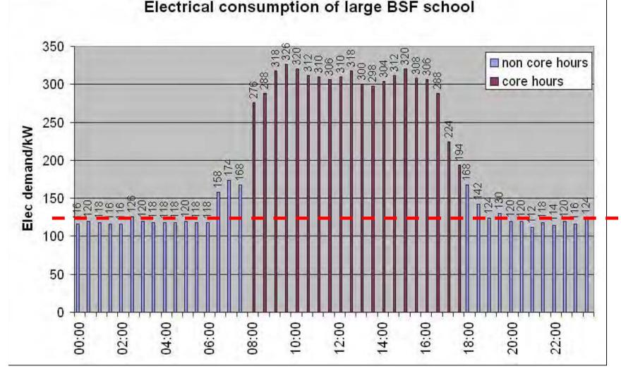
120 kW baseload: ca. 7 W/m<sup>2</sup> or 45 kWh/m<sup>2</sup> p.a. Equivalent to 60% of all lighting or 1000 PCs including screens. printers etc.
