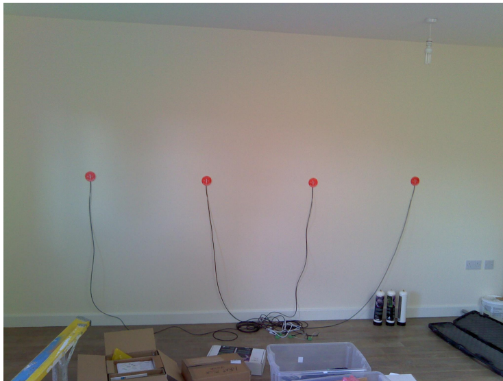
Photo 12 Heat flux sensors on living room party wall
