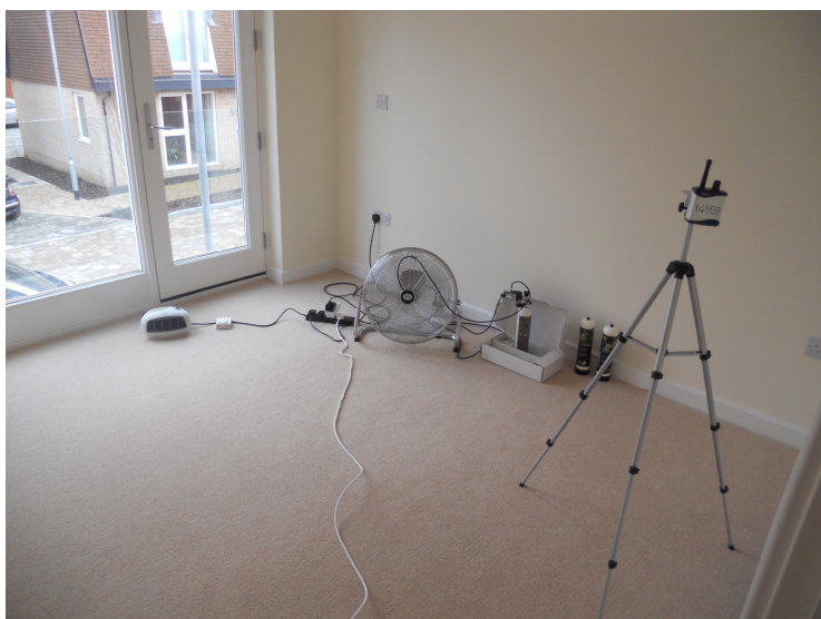
Photo 5 Co-heating test equipment in Bedroom 2
