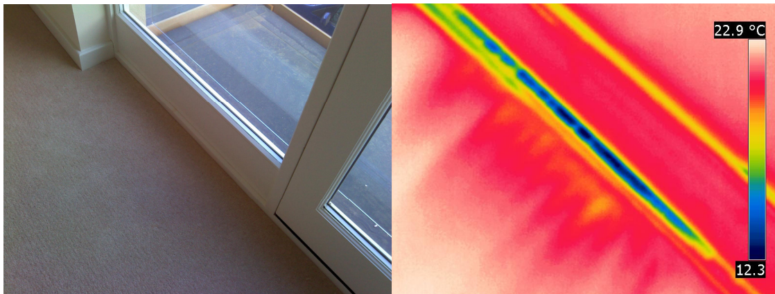
Photo 9 Air leakage under Bedroom 2 glazed panel
