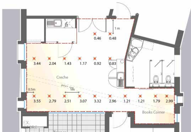
Fig 5.8.3 - First Floor Crèche Daylight Factor (%) mapped onto plan of room – showing a better level of uniformity than achieved on the ground floor.
