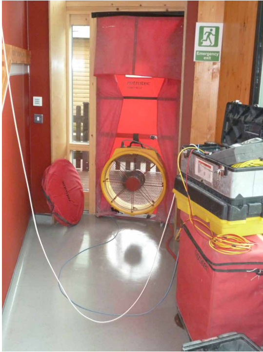
Fig.5.12.2- photo of the air pressure testing equipment installed.
