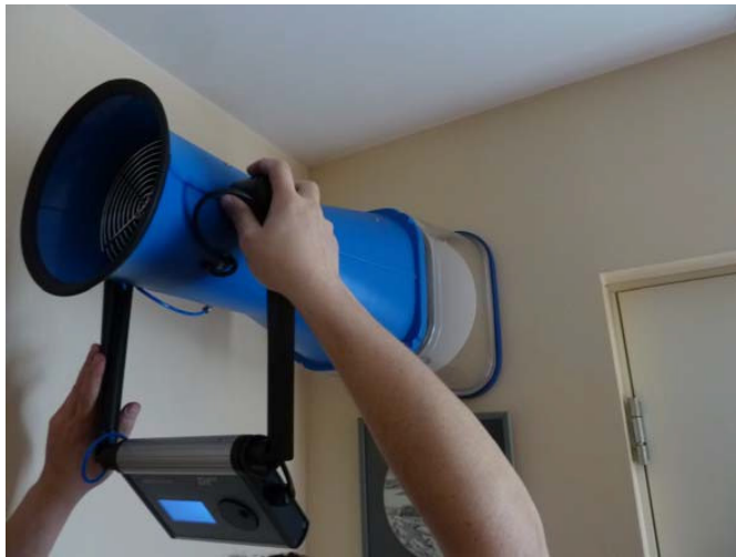
Fig 9.1: Powered flow hood in operation showing volume flow rate of kitchen fan
