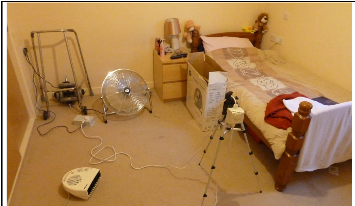
Co-heating kit disposition in one of the test bedrooms
