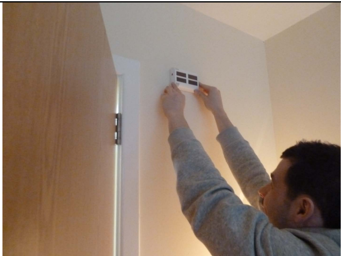
Fig.8.1 A wireless temperature, relative humidity and carbon dioxide concentration monitor. These units are less intrusive than other monitoring kit and also benefit from operating using solar power and battery backup.
