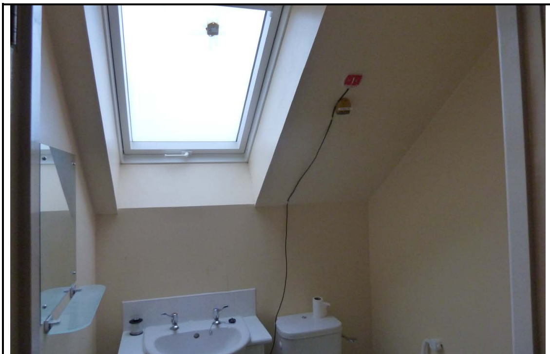
U-value kit sensor arrangement testing the heat transfer through the roof. Unfortunately the flux plate in this location became dislodged during the test.
