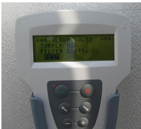
Figure 7.16: Dirty air filter alarm
