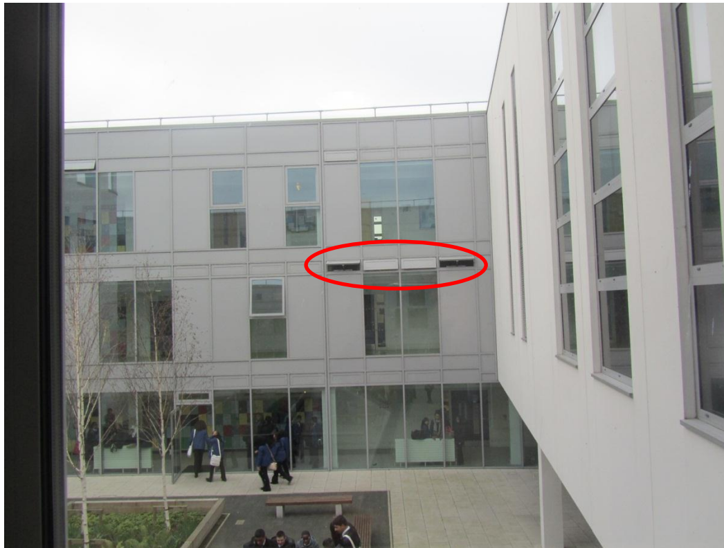
Figure 6.4: Motorised vents stuck open regardless of CO 2 level and temperature, Classroom F21 (Photo taken on 15/01/2013)
