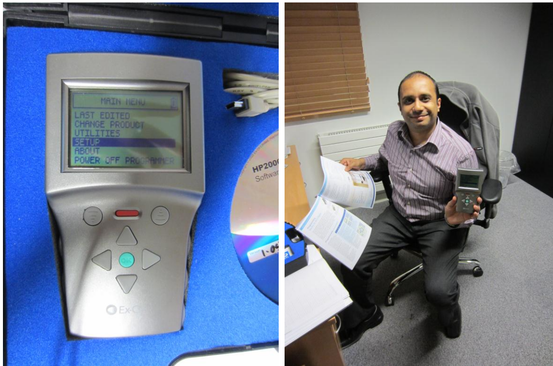
Figure 3.4: Handheld device for programming all the school's lighting sensors and their zoning found by IT manager in a box two years after the building opened.
