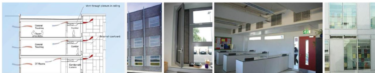
Figure 3.1: Plenum ventilation strategy of classrooms showing windows, plenum vents and courtyard flaps
