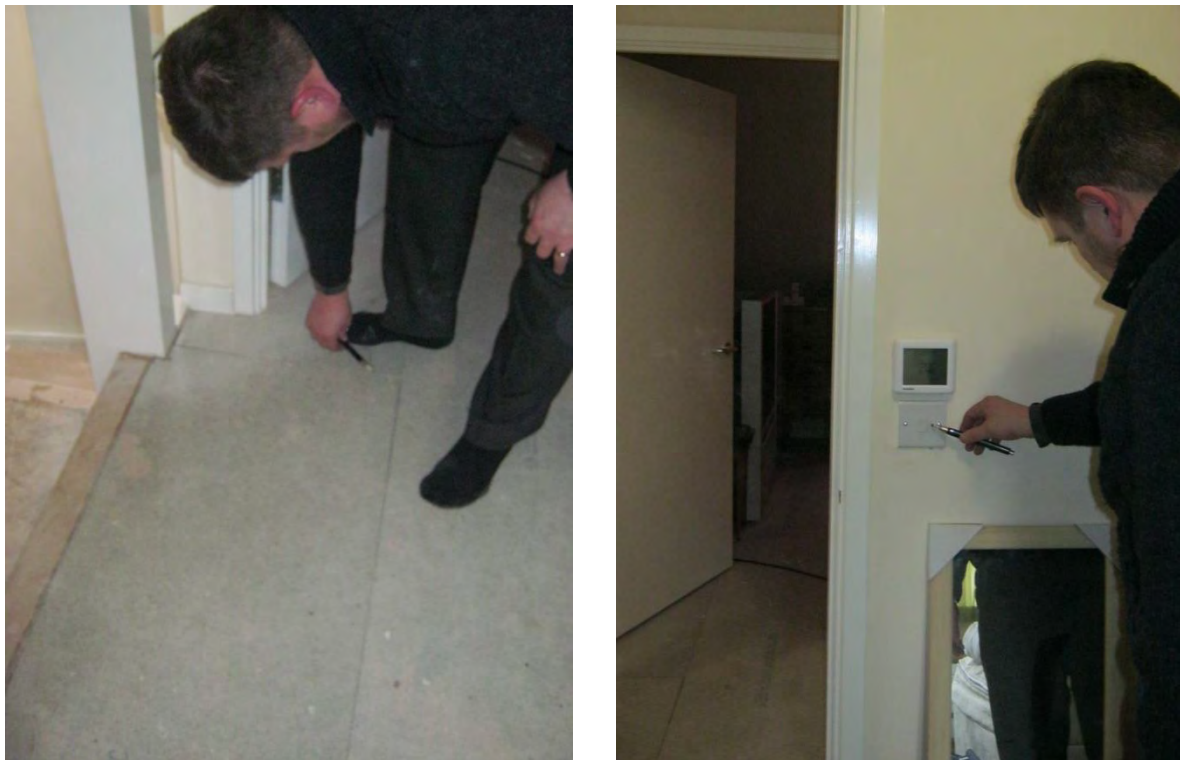
Figure 53 Smoke pencil test
