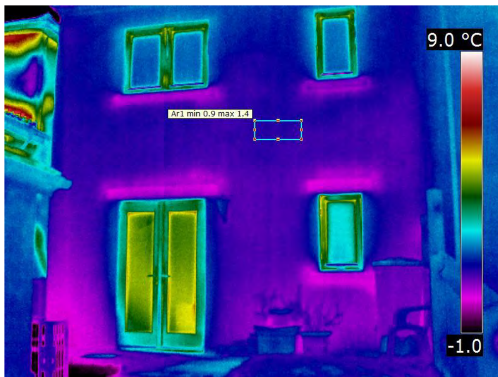
Figure 24 No.1 rear (west) elevation thermogram. Note: No thermal abnormalities are evident in the walls.
