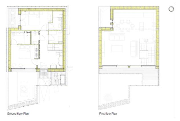
There is a heavyweight concrete wall around the back (north-east) and sides of the house, with the main glazed elevation facing south-west.
