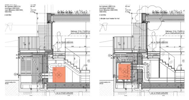
These sections show how the air handling unit for the MVHR was moved from under the stairs (left) to the cycle store (right) to improve access to the filters.
