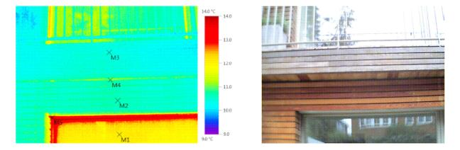
The only significant area of heat loss is the perimeter of windows – the frames and window reveals were 14  $^{\circ}$ C.
