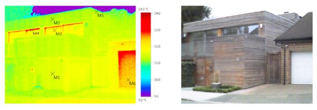
There is minimal heat loss through the walls – although surface temperatures are very low because of the air gap behind cladding
