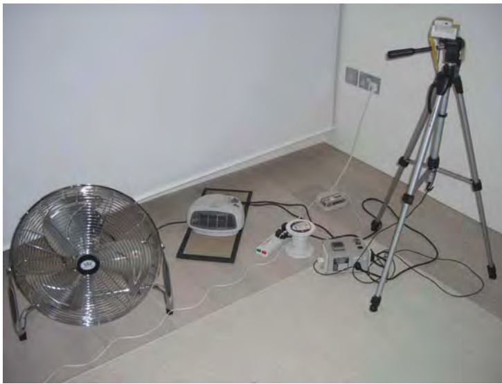
Figure 3-3. Camden Passive House: co-heating test equipment
