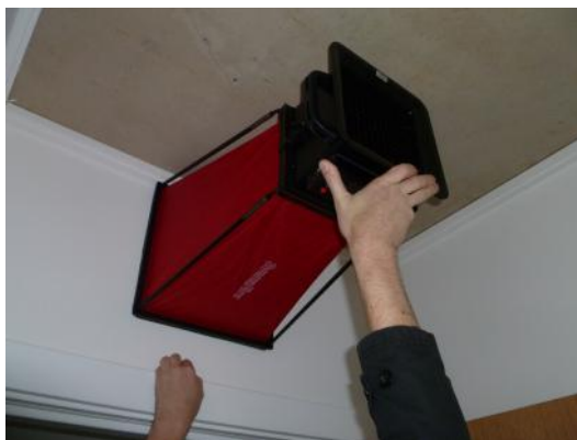
Figure 15 MVHR duct grille flow measurements undertaken using a Swemaflow 125D.
