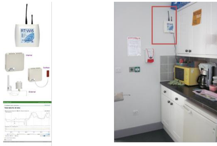
Figure 84 Left: The Wi5 data hub, the Internal Temperature/Humidity and CO 2 transmitters and the external temperature/humidity transmitter. Right: One of the two data hubs was placed in the 3rd floor kitchen.
