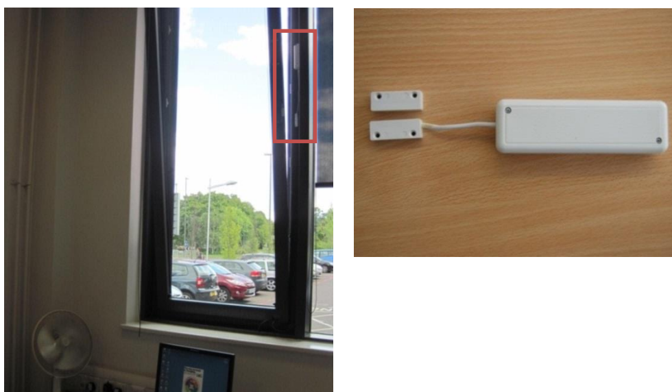
Figure 87. Left: Windows opening and closing activity sensors were placed in the windows to monitor the use of the openings during summer and winter season. Right: Window sensor.
