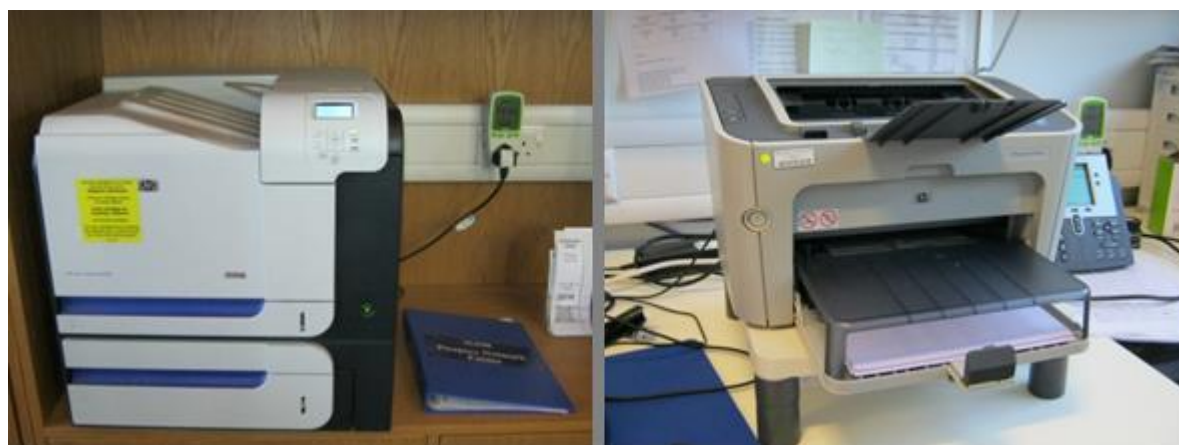
Figure 136 Measure of key equipments' energy consumption using true power meters.
