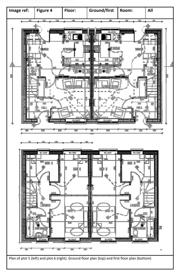
Timber frame panellised system using on-site modern methods of construction (MMC) were employed. External facades use cedar panelling or brick with blockwork in the inner leaf separated by an insulated 75mm cavity. Suspended floors consisting of timber joists and chipboard are used. The roof consists of integrated modular PV panels and tiles with 200mm of mineral wool insulation between the joists and a further 200mm on top (400mm total).
