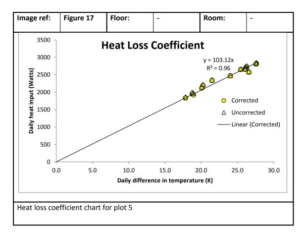
daily wind speed throughout the test period was only 0.94 m/s, the daily solar flux averaged  $91 \text{ W/m}^2$  (building is a timber frame with a low thermal mass so these results are unsurprising).
