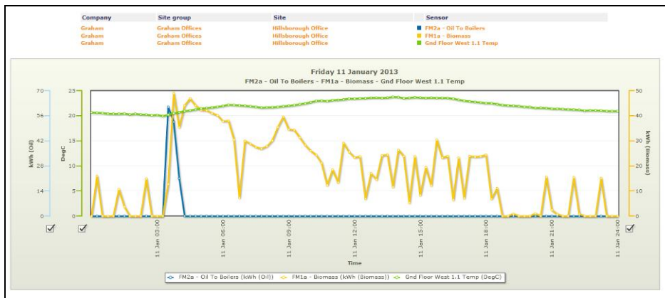
Figure 7.34 Boiler load profiles January 2013
