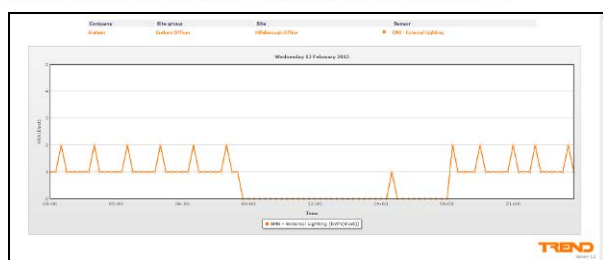
Figure 7.13 February 2013 –Lights on all night –fault in timer
