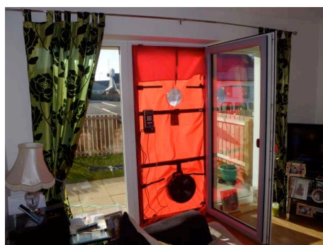
Figure 5 Pressurisation test being undertaken on the extensively monitored dwelling.
