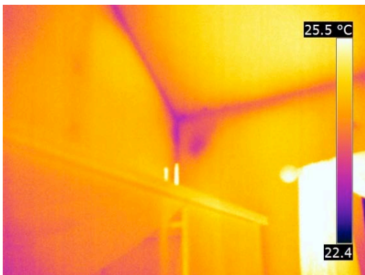
Figure 12 Spot on the external wall of dwelling 7.
