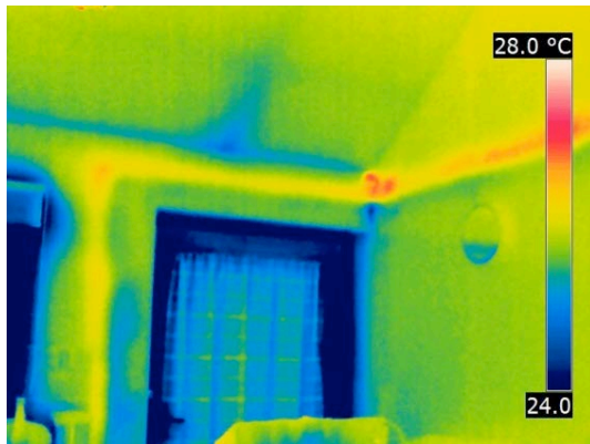
Figure 11 Strip running across the partition wall and above the back door in dwelling 2.
