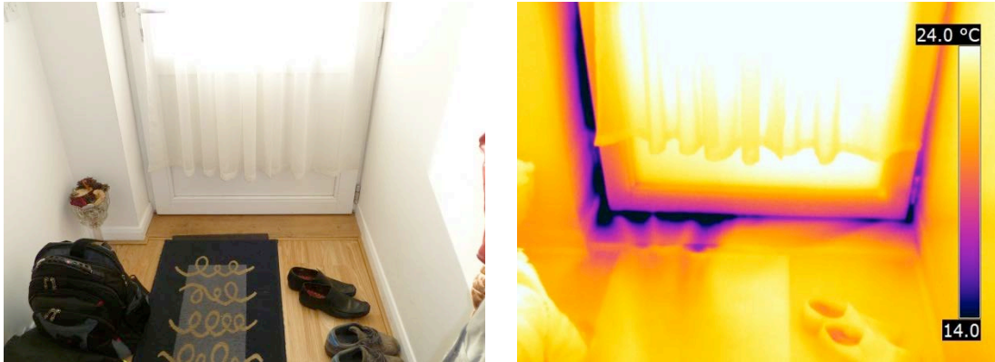
Figure 8 Leakage at the bottom corner of the front door.
