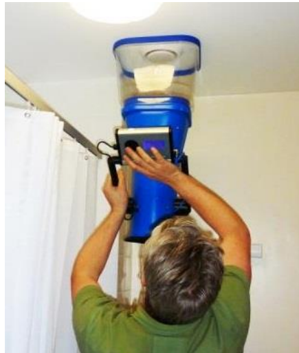
Figure 60 MVHR testing. Measuring the extract rate in the bathroom vent.
