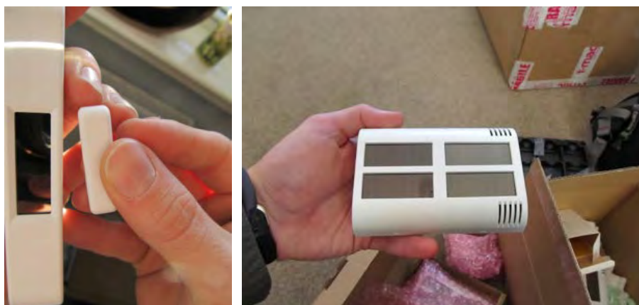
Figure 53: Window contact sensors (left) and combined CO 2 , temperature and RH sensor (right).
