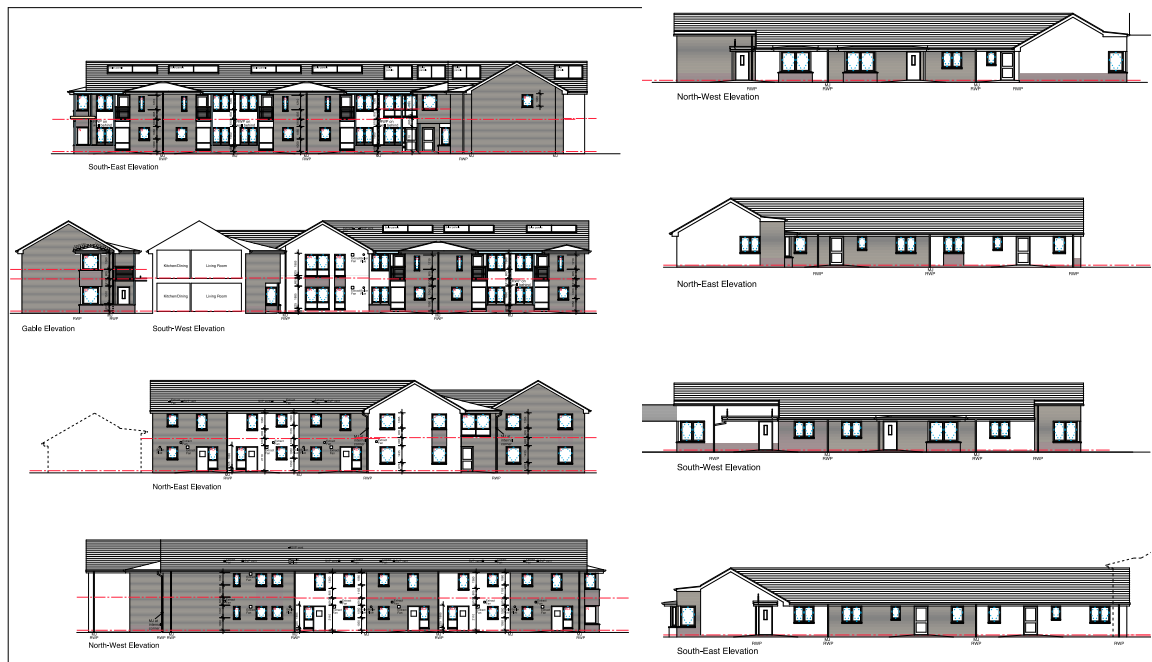
Figure 9: South elevation - note 2 solar panels on the roof of BB1 (left); North and east elevations - note reduced window sizes (right)
