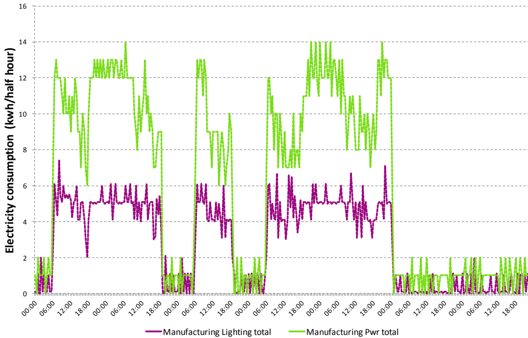
Figure 6.10: NCC - Weekly electricity profile for 20 th May 2013 to 26 th May 2013 showing manufacturing lighting and manufacturing power submeters consumption.
