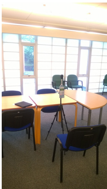
Figure 3: Internal sound level meters in open plan office on the ground level – windows closed
