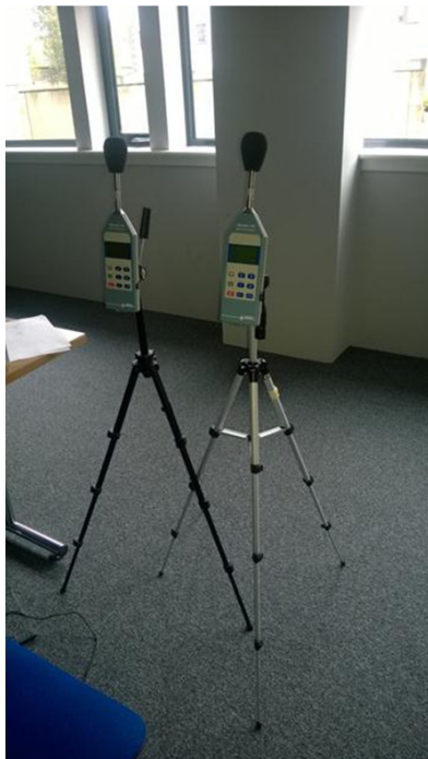
Figure 1: Two sound level meters ready to take measurements after calibration
