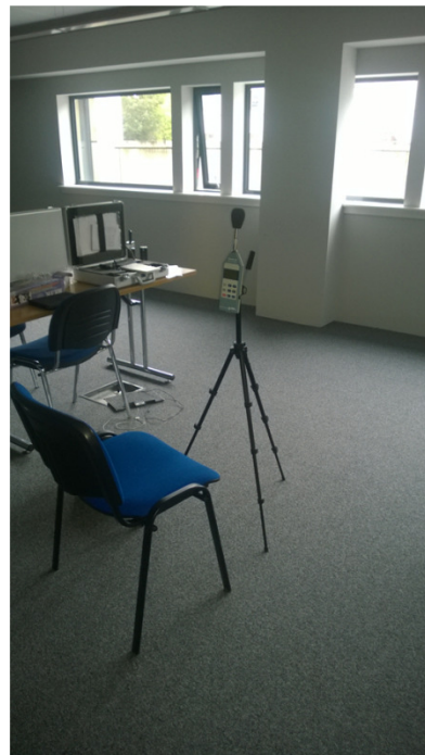
Figure 2: Internal sound level meters in open plan office on the ground level – windows open
