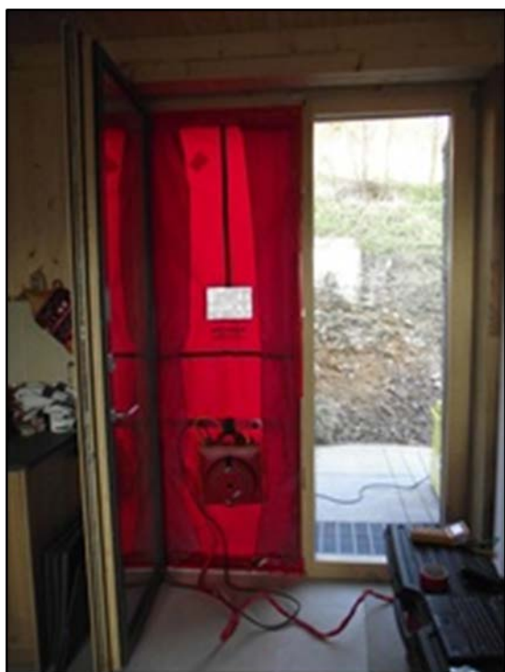
Picture 21: Test equipment mounted in side door
