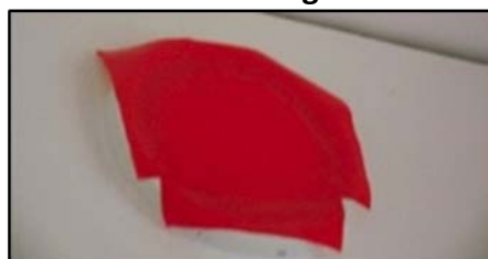
Picture 22: Hit-and-Miss vent closed for duration of testing
