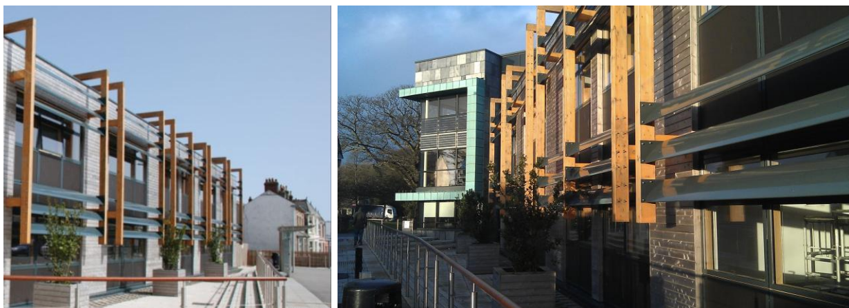
Figure 9 Brises soleil on the south-east façade
