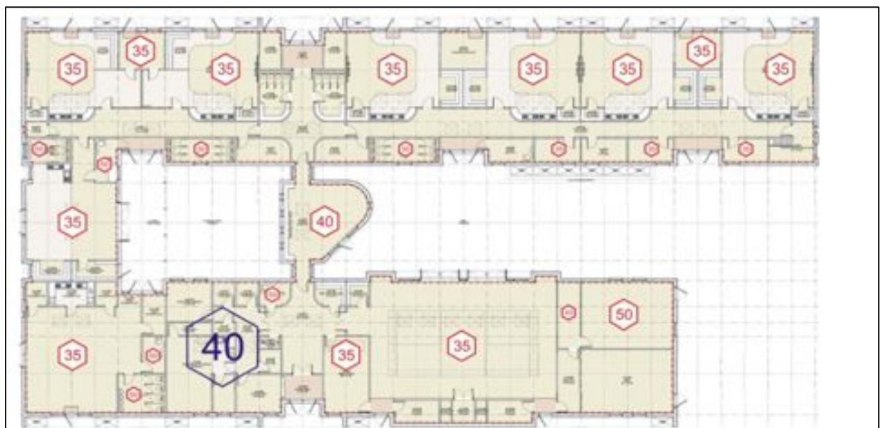
Figure 2.2 : Recommended maximum ambient noise levels(db) in spaces throughout the building.
