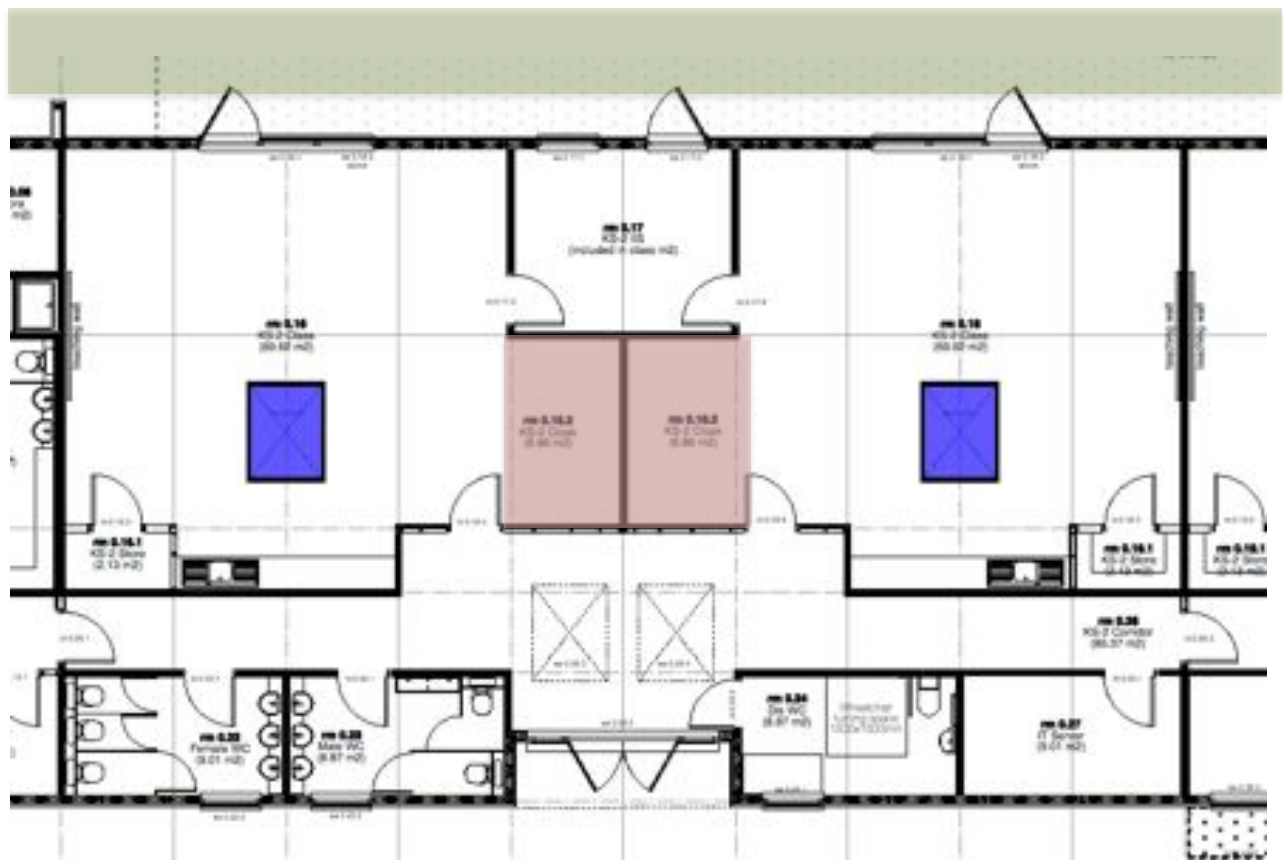
Figure 2.4: Classroom layout: roof light location (blue) and area opened up to the class-bases (pink)
