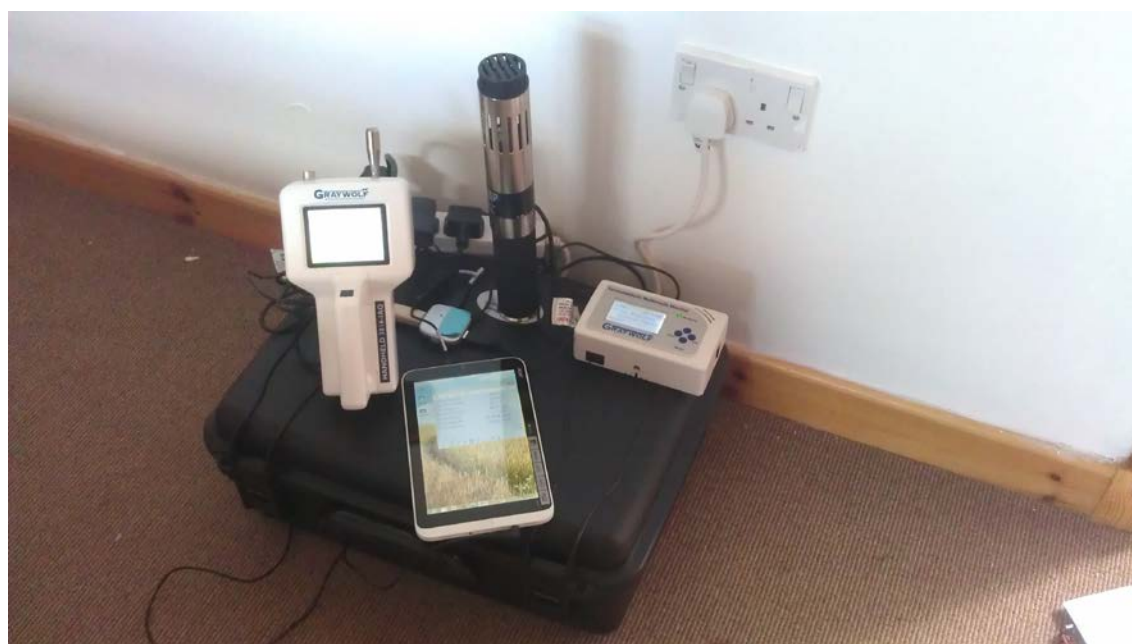
Figure 8:1: Portable VOC monitoring apparatus in dwelling B1.
