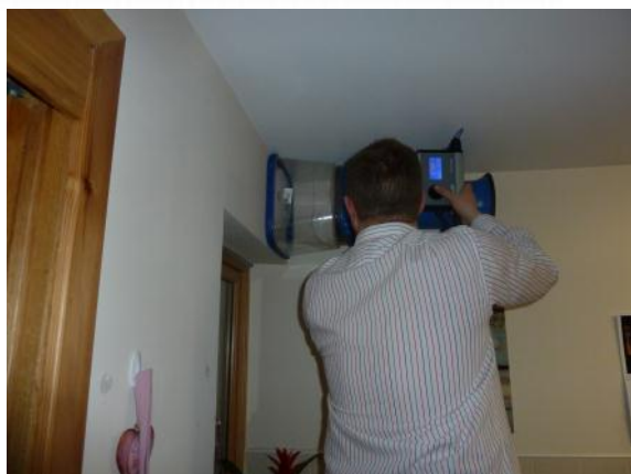
Figure 6:9: Flow measurement testing in kitchen, dwelling D2. Note how the apparatus just fits.
