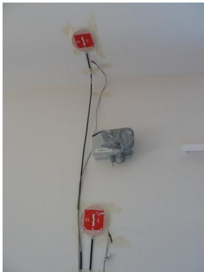
Figure 3:3: 2no. Hukseflux HFP01-10 heat flux plates (red discs) and ambient air temperature sensors (short black objects) installed beside each HFP. The HFP and temperature sensors are wired to two Eltek GenII, type GD-32, thermistor input transmitters. An Eltek GenII, type OD-12, external thermistor input transmitter is located internally as a back-up should an ambient air temperature sensor become loose and fall.
