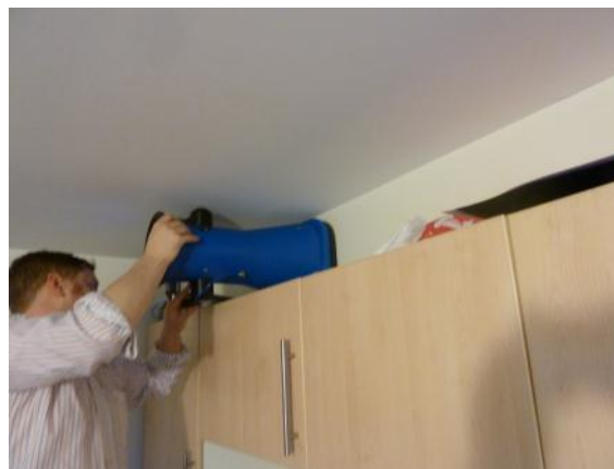
Figure 6:8: Flow measurement in kitchen, dwelling C1, access to grille above wall mounted cupboards with measurement apparatus was difficult.
