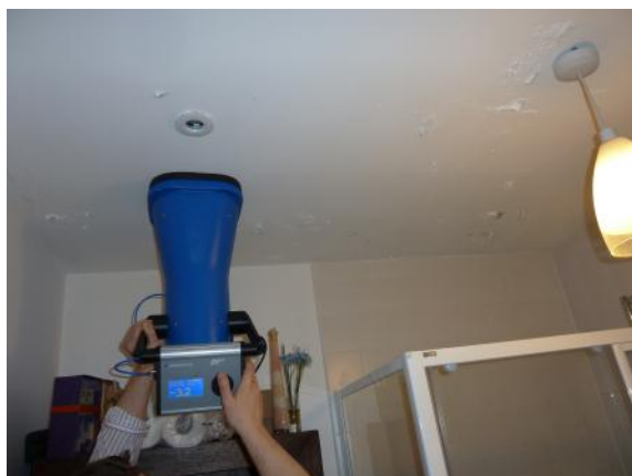
Figure 6:1: Volume flow measuring equipment (without extension hood attachment) in ground floor bathroom in A2. Note extent of peeling decorative paint.
