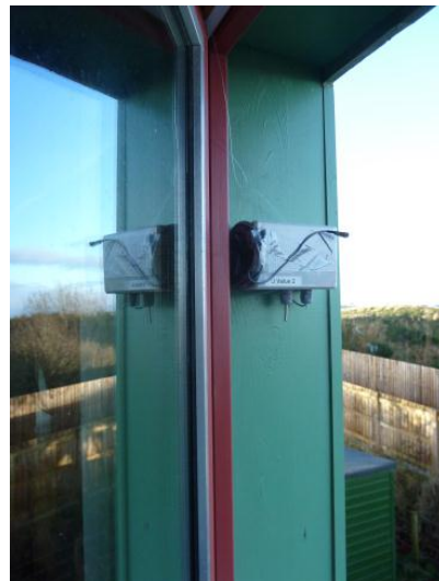
Figure 3:4: Eltek GenII, type OD-12, external thermistor input transmitter.
