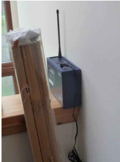
Figure 3:1: Eltek Squirrel 1000 series, type RX250AL, Radio telemetry data logger set up on a landing.
