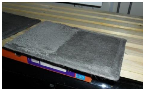
Figure 6.8: The extract side filter partially cleaned to illustrate the before-after change
