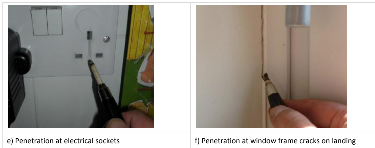
Figure 3.1: Photo evidence showing areas of air leakage penetrations around the Flats
