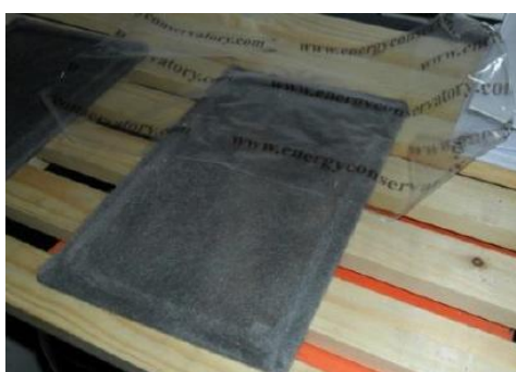
Figure 6.9: Tape being placed across 50% of the filter to simulate a 50% blocked filter
