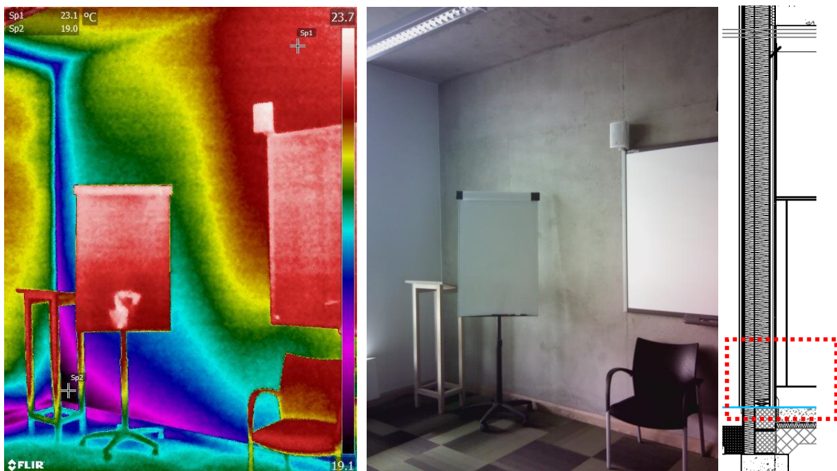
Figure 7.10 Interior of southwest facing external wall in the Catalpa room (directly below the Walnut room). Thermal abnormality where the exposed concrete wall and ceiling meets the wall plaster on the interior of the external wall; \sim 4^{\circ}\text{C} difference between the lowest point on the adjoining concrete wall (Sp2) and highest point toward the interior of the room (Sp1).
