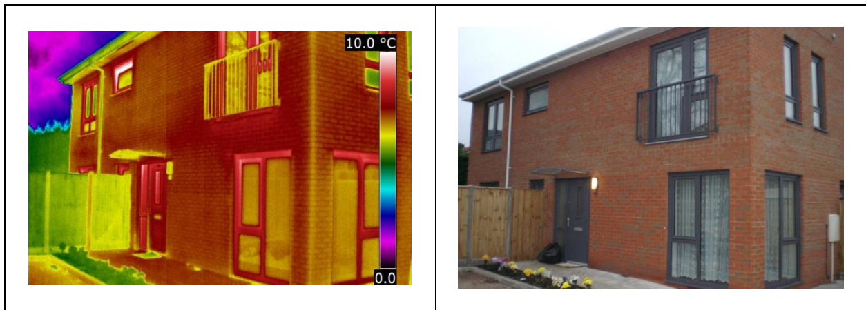
Figure 15 (Left) Front elevation thermogram. Note: No thermal abnormalities are evident in the walls. The elevated temperatures of the window surrounds and the front door is likely to be due to the change in material, whilst the elevated temperatures in the upper centre bathroom window could either be due to poor fitting or simply that the window has been left open. (Right) Front elevation digital photograph.
