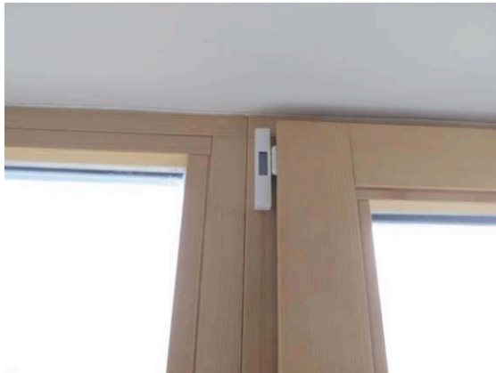
Figure 7.1: Window contact sensor: closed.
