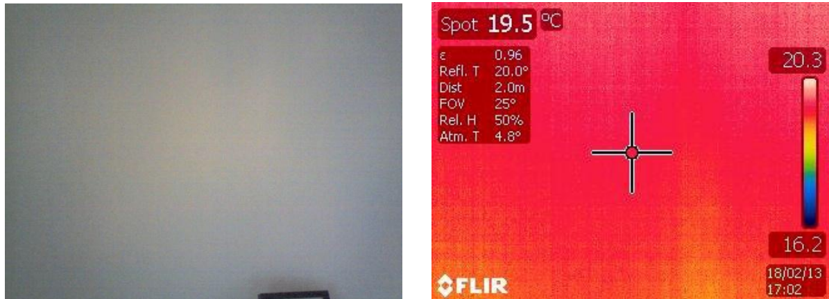
Figure 3.1: Thermographic imaging before mounting of heat flux sensors to ensure sensors are mounted on a surface representing even thermo physical properties in dwelling TB1.
