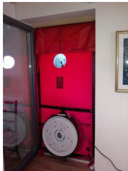
Figure 3.5: Air pressure test door fan in TB1.
