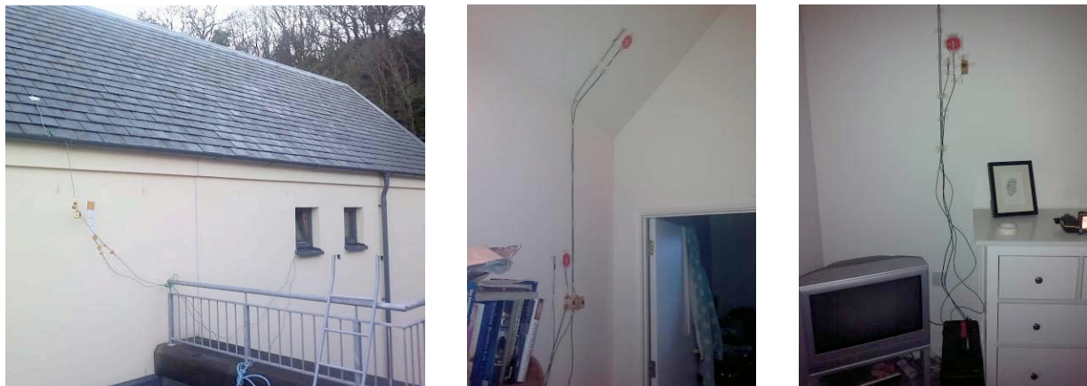
Figure 3.2: Air temperature and Heat Flux sensors mounted on internal wall surfaces in dwelling TB1.
