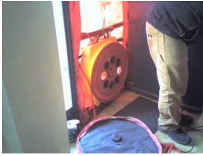
Figure 3.3: Air pressure test door fan in Dwellings TA1 and TA2.
