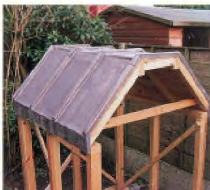
Figure 13 This outdoor test rig near Manchester has 100% outside air ventilation. Little ULC has been found here, apart from an area of the flat central section above which a shallow puddle of rainwater collects.
