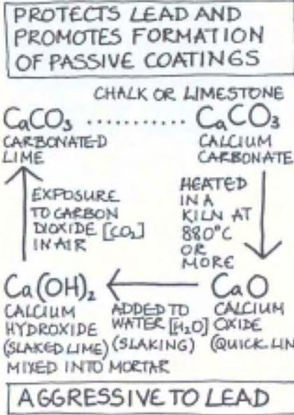
*Figure 11 The lime cycle. Calcium carbonate –  $\text{CaCO}_3$  – the start and end point of the cycle, is nearly neutral, does not attack lead and can help to protect it. Slaked lime –  $\text{Ca(OH)}_2$  – is alkaline and aggressive to lead.*
