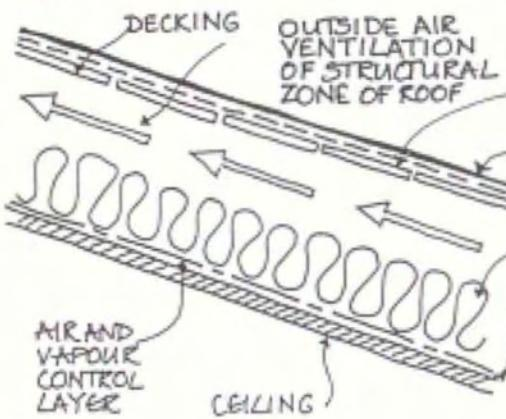
**Figure 3** The cold deck roof (left) and ventilated warm roof (right) are similar in principle. Ventilation should be by outside air only, and run from bottom to top with no dead spaces. For good performance, the air and vapour control layer (AVCL) must be both air and vapour tight. This is much more easily done in the VWR, where the AVCL can be applied on top of the structure. In an existing building it is very difficult to install an effective AVCL at ceiling level.
