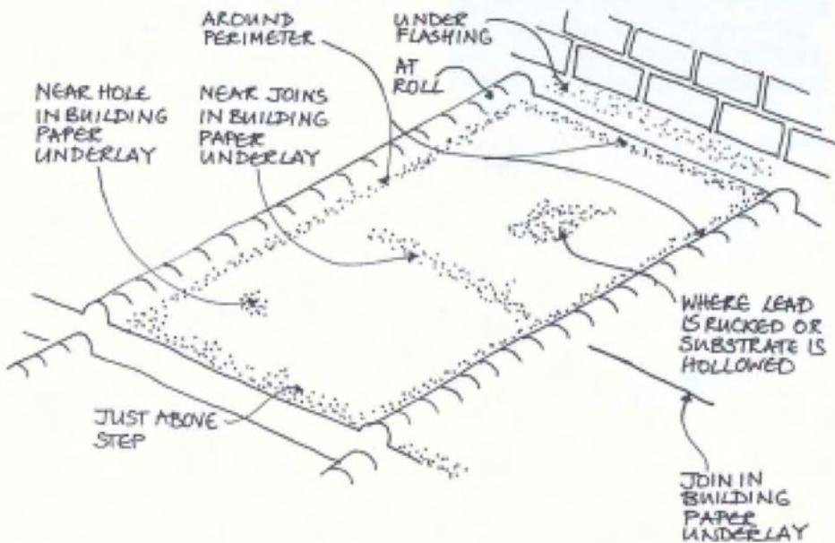
*Figure 10 Typical locations of acid-related corrosion. If acids are present, corrosion is often found around the edges of the lead sheet: inside rolls, above laps, and above areas where the lead has become blistered or folded, or the substrate dips away. This appears to be a consequence of distillation of water across the air gap, easier access of carbon dioxide to regenerate acid from the lead salts, and electrochemical effects.*
