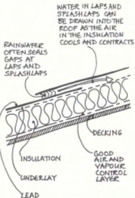
**Figure 4** Warm roof construction should not be used because water or moist air can be drawn in as the roof cools down.
