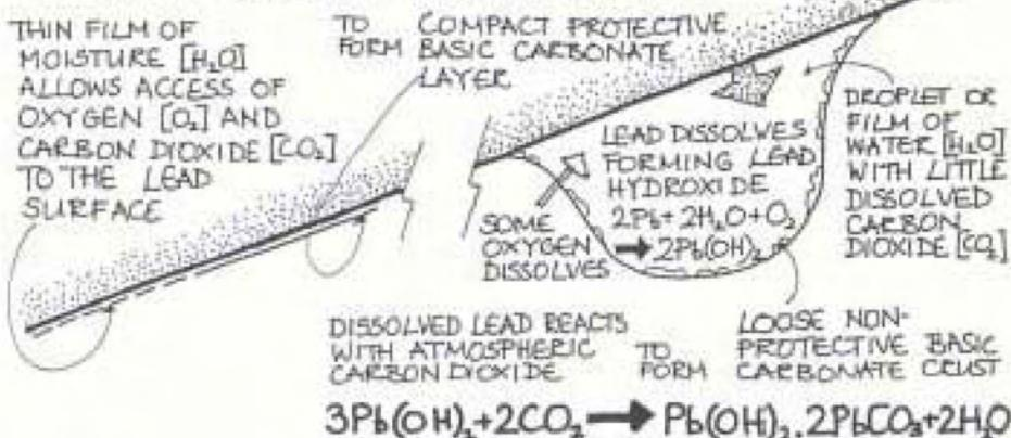
Figure 6 Where reaction with a thin film of water, oxygen and carbon dioxide occurs at the surface of the lead (left), a compact film of basic lead carbonate (often also containing lead oxide) can build up. This can help to protect the lead from further corrosion. On the right, however, carbonation occurs at the surface of a water droplet, and this forms an unprotective powdery or flaky crust.
