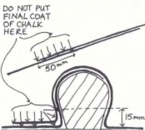
Figure 31 Do not put chalk at the very edges of the sheets. It could draw in moisture.
