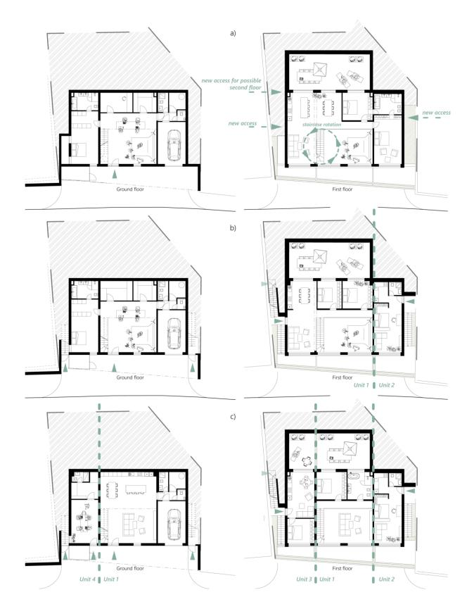
**Fig. 4**. Adaptable house NO.2 – villa with a studio for a photographer and his family. The evolution of the design shows a) a preliminary solution with operation enabling adaptability. Adding access points and rotating the staircase enables the future division and different use weight of the rooms or units; b) and c) new access points and polyvalent staircase can divide the house up to 4 independent units. (Source: Lüley in cooperation with Eckhardt studio, 2023)
