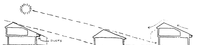
Diagrams of site layout and spacing between terrace based on maximum solar penetration and economic district heating runs.
