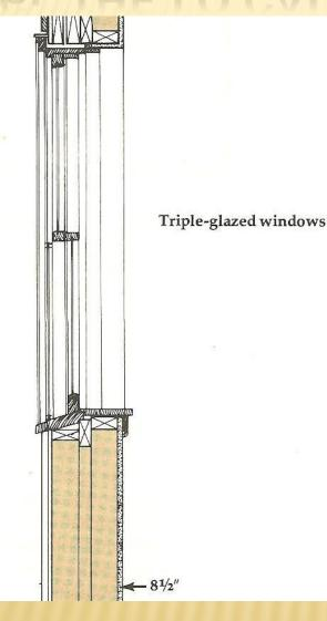
× Long axis of the house is oriented east-west. × Double 2x4 walls (R-30) × R-33 ceiling x Triple-glazed windows × An air-to-air heat exchanger
