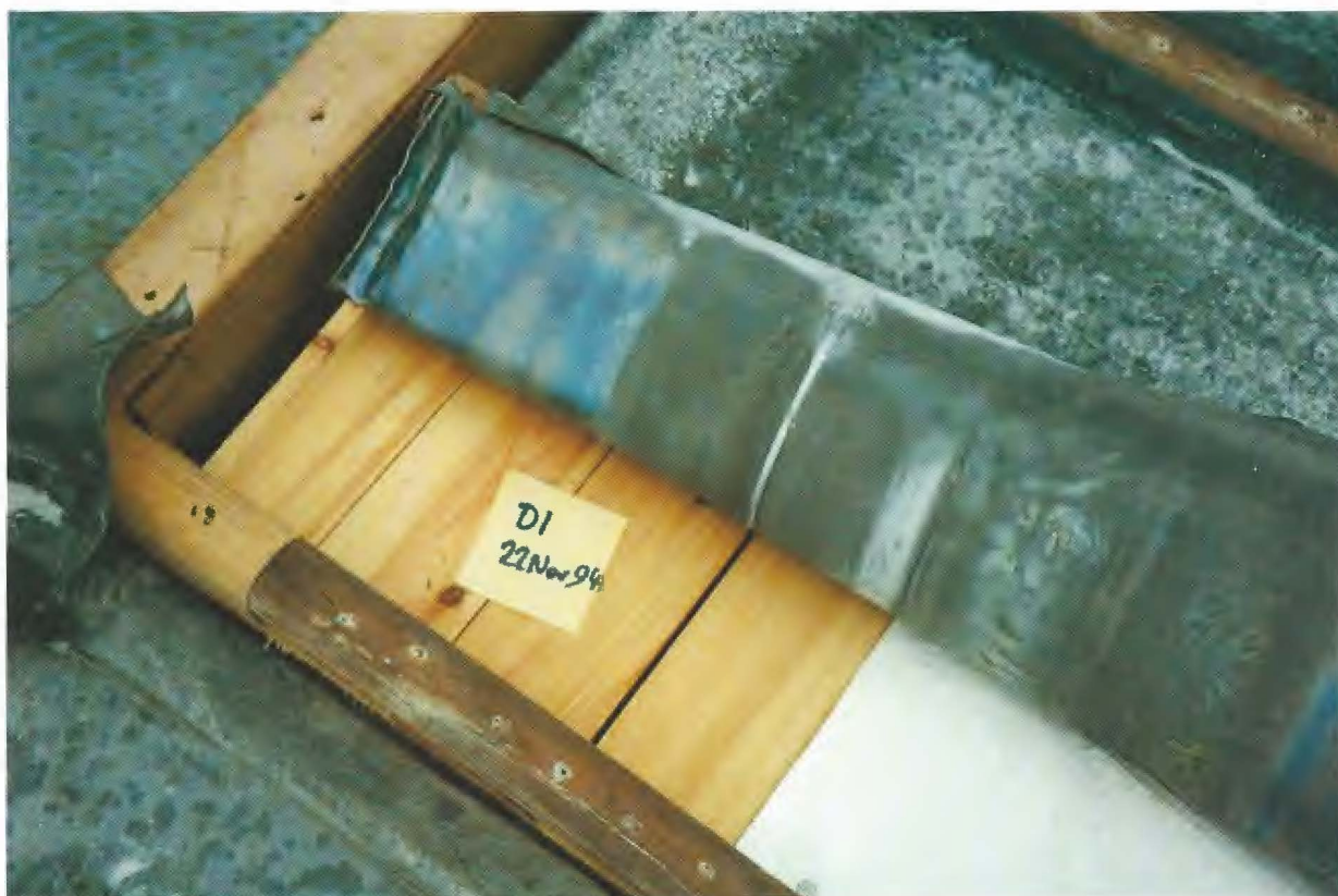
Plate 3. Lead after a two-month autumn test at Donnington Castle showing a wide range of surface states from passivation to corrosion. The two (untreated) boards on the left have kept the lead dry and its underside is only slightly dulled. The two to their right were preservative-treated and probably initially damper. This has assisted passivation over much of the boards, but corrosion around the perimeter. See also Figure 7, p 39.
