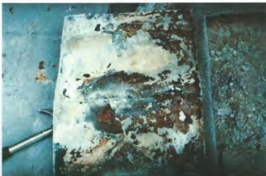
Plate 10. Underside corrosion over oak at Norwich Cathedral cloisters. The patch removed, on the left, failed at the perforation in the middle. The characteristic red/brown oxide can be seen near the interface with the metal, with the thick, flaky and granular corrosion product remaining underneath (on the right). See also Figure 19, p 44.
