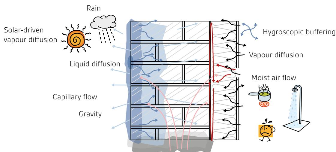
4. Moisture problems occur mainly at the junctions between elements and the interfaces between materials. Any approach to moisture risk which does not take this into account is inadequate. These effects are called *connective effects* in this document.
