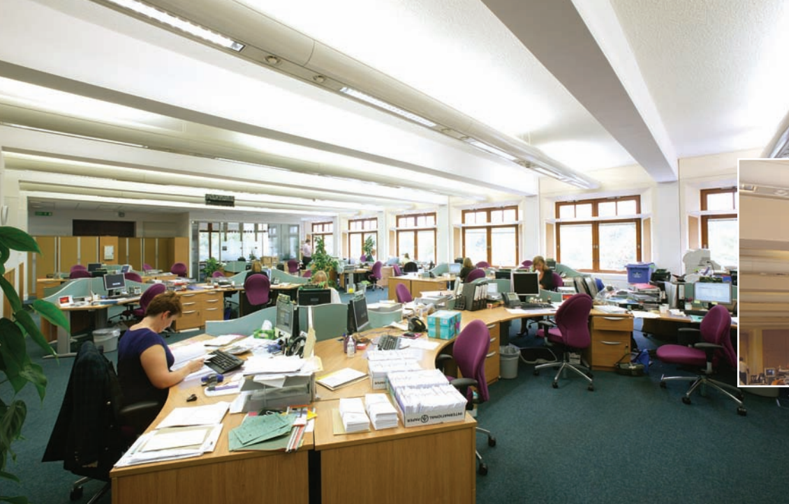
LEFT: The introduction of flush floor trunking runs have freed up the layout in the refurbished offices ABOVE: Uplighters, providing only patchy lighting in the building before its refurbishment, were the basis of one of the occupants' complaints
