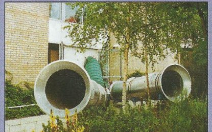
The BREFAN unit was also operated in reverse to de-pressurise the building and enable smoke tubes to identify the paths of air leakage.
