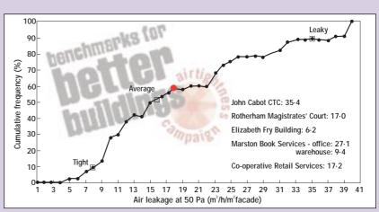
FIGURE 4: The air leakage data for the CRS headquarters building, plotted on the BRE/BSRIA database.
