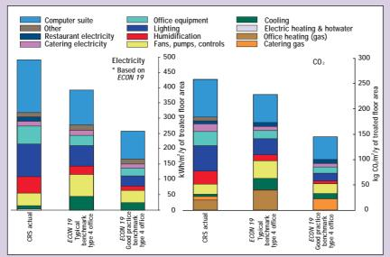
FIGURE 1: End-use energy breakdown at the Co-operative Retail Services headquarters building. The conversion factors are: gas – 0.2 kg C0 $_3$ /kWh and electricity – 0.52 kg C0 $_3$ /kWh.
