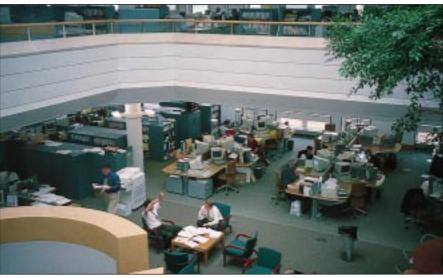
The ground floor offices at Co-operative Retail Services, viewed from an atrium. Due to the unreliable lighting control system, the metal halide uplighters tend to be on outside of normal office hours, contributing to an 'uplift' of 3-4°C to the supply air temperature in the first floor plenum.
