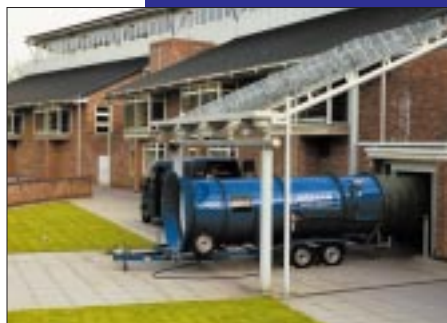
The BREFAN Large Fan Pressurisation System during the BRE pressure test at the Orchard Learning Resources Centre.
