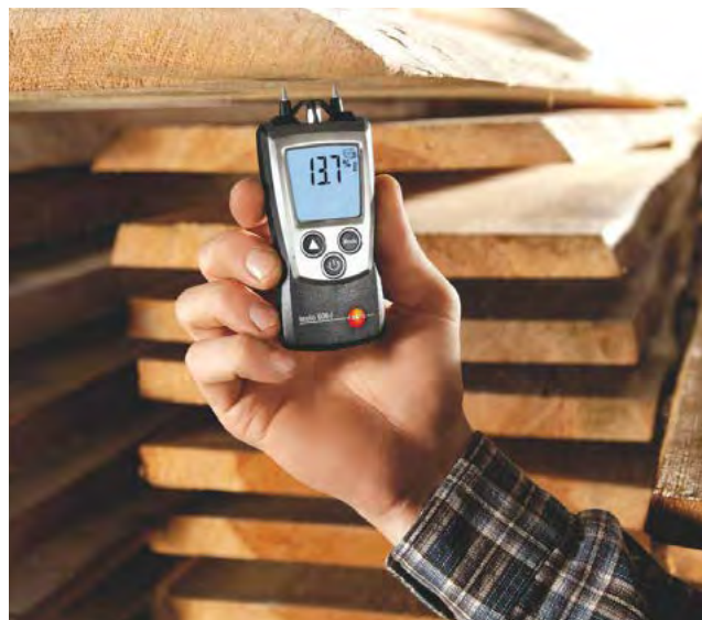
Illustration of moisture strategy checks during the construction stage: Example of 2-pin capacitance moisture meter being used on timber before it is installed; this is a common type of moisture meter for this type of application. (Source: Testo)
