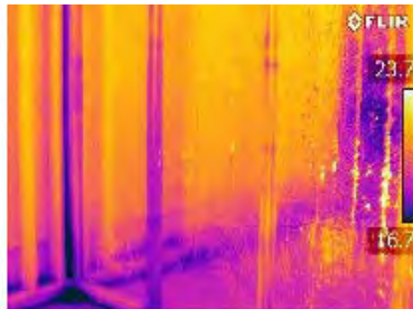
Thermogram 1 illustrates the overshadowing effect of the high reflective coating of the insulation
