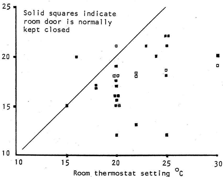
Figure 2. Relationships between measured and thermostat reading in sitting room
