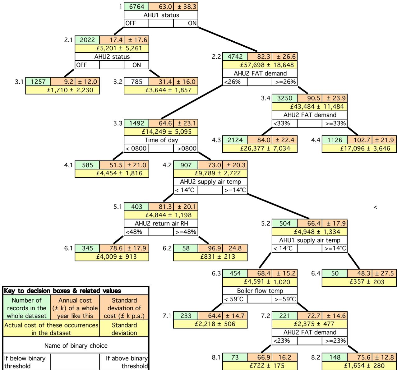
**FIGURE 1: DECISION TREE FOR THE TWO MAIN AIR HANDLING UNITS IN THE OFFICE MONITORED**
