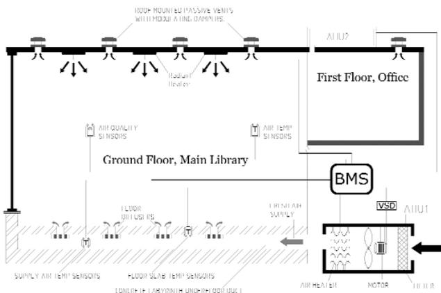
Figure 1: Environmental Control System - Overall Concept
